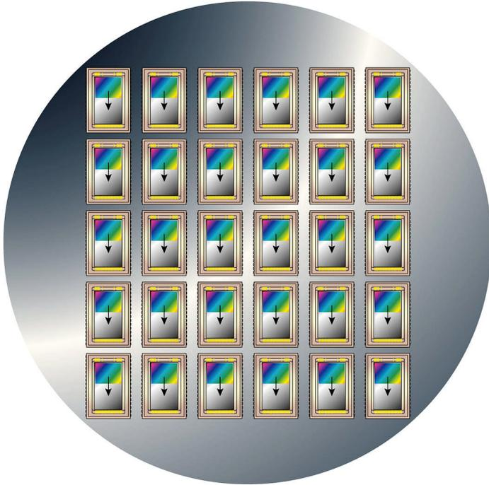
Figure 5: A schematic of how an array of EMCCDs might be arranged to allow coverage of wide fields of view.
