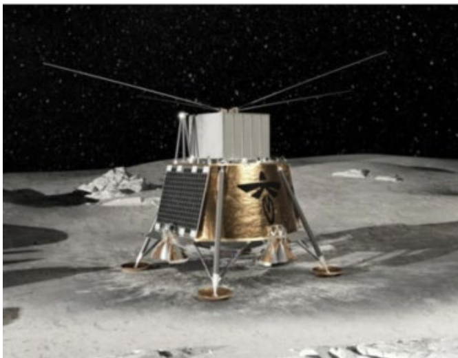
Figure 1.: Proposals for observations of the dark ages 21-cm signal focus on missions to the Lunar surface or to Lunar orbit. The figure shows one such experiment called the Lunar Surface Electromagnetics Experiment-Night (LuSEE-Night) which is being developed by NASA, University of Colorado Boulder and the USA Department of Energy and is set to launch in late 2025. Correctly interpreting the results from these experiments is crucial if they are to be successful and that requires projects like this one to help us better understand the physics of the early Universe.
