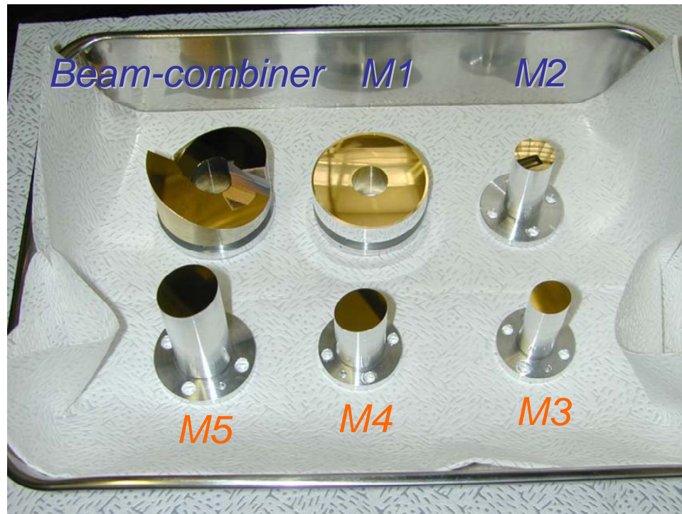
Optical component (deposited by Cr and Au)
